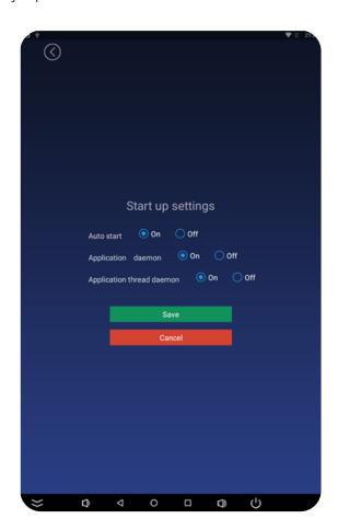
When you are planning to deploy the device, set all three options to On. This lets the device monitor the application, to ensure it's always running at any point in time.
