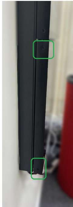
Where to unscrew & secure mount
