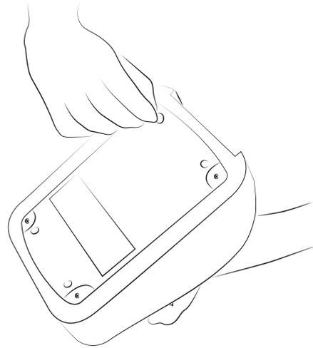
14. Remove the feet on the bottom of the badge printer. These may be glued on so may be difficult to remove
