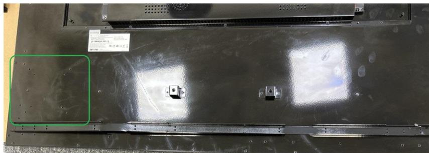
Area where mini PC can be mounted on the back of the display
