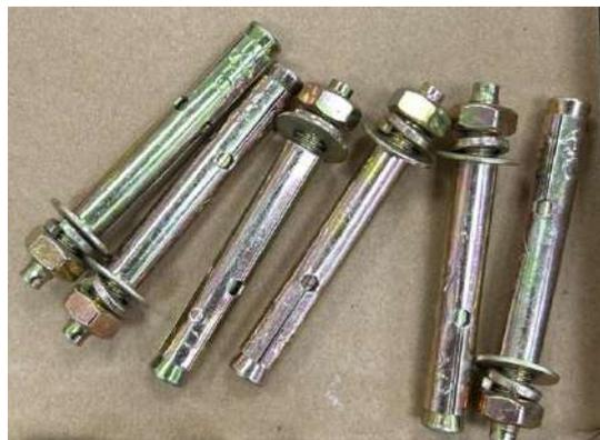
Anchor bolts for mounting the frame onto solid walls
